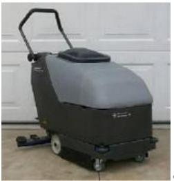
Our company also owns floor equipment such as our Advance Micromatic auto scrubber. This one is so good at cleaning larger floor areas such as in lunchrooms and the larger rest rooms. It scrubs and then vacuums the dirty water up leaving the floor surface much cleaner than when just using a wet string mop.
